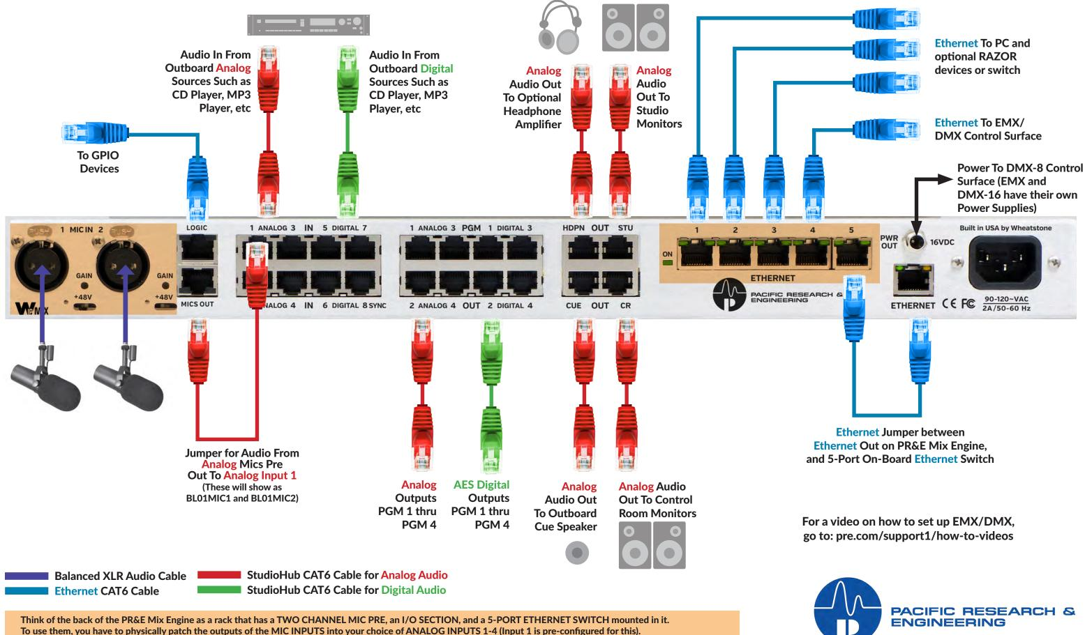
To use them, you have to physically patch the outputs of the MIC INPUTS into your choice of ANALOG INPUTS 1-4 (Input 1 is pre-configured for this). Likewise, to use the PR&E Mix Engine with the 5-port switch, you need to physically jumper the ETHERNET OUT to an available port on the onboard 5-port **ETHERNET** switch.
